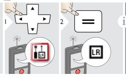
The long range mode allows measuring of difficult targets in unfavorable conditions e.g. bright ambient light or bad target reflectivity. The measuring time is increased. An icon in the status line shows if the function is active. EN
