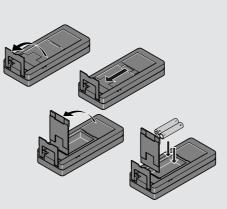
To ensure a reliable use, do not use zinccarbon batteries. We recommend using high quality batteries. Change batteries when battery symbol is flashing.
