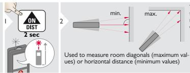
The minimum and maximum distance measured is displayed (min, max.). The last value measured is displayed in the main line.
